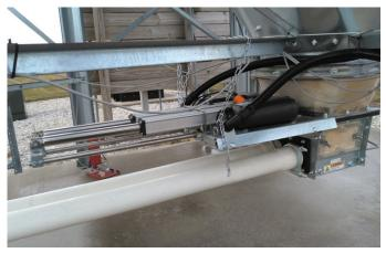
Single or twin options are available. Automatic opening based on load cell, or proximity switch inputs.
